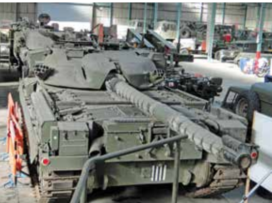
ABOVE LEFT: This is the final version of the Chieftain, a Mk.11 with its Stillbrew armour around the front of the turret and TOGS gunnery system in place of the searchlight. The front part of the Chieftain turret was made from cast steel with some large tolerances, so the Stillbrew package had to be custom made for each vehicle. ABOVE RIGHT: A Scammell Pioneer tank transporter and an Austin gantry breakdown vehicle beautifully restored to show them as used in the Western Desert of Africa during WW2.
