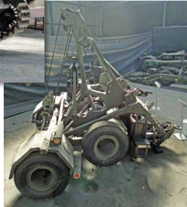
RIGHT: This is a very rare beast indeed. It's an FV3561 Dummy Axle 10-30 tonne Recovery Trailer. It could be attached to a Thornycroft Antar tractor unit to enable it recover a disabled one by lifting up the front axle to have a suspended tow. It is similar to a smaller 1-3 tonne version.
